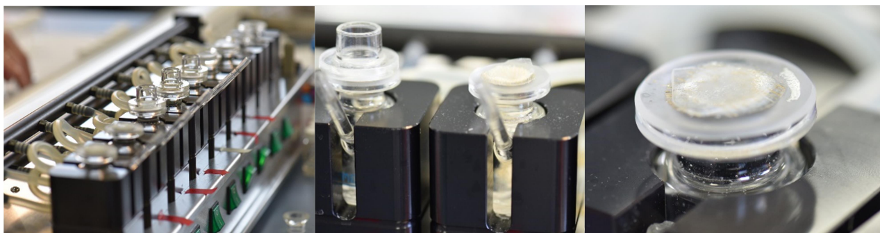
Franz cell setting for a polymeric film on a porcine skin biopsy
